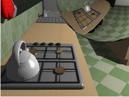
Figure 13: Example of Z-fighting when a small object is layered on top of a larger object.
