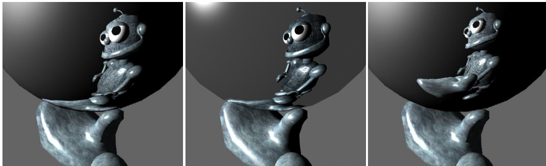
Figure 1: Left: Specular reflections computed with our algorithm. Middle: ray-traced reference. Right: Environment map reflection.
