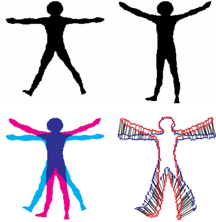
Figure 6. Matching results of human body with different hand and leg positions. [Top row] Silhouettes of two difference human bodies. [Bottom row] (left) Superimposed images of the two human body silhouettes. (right) Correspondences. In this matching experiment, three scales \sigma = 12, 10, 7 are used in a coarse-to-fine manner and \alpha = 0.0005 , \mu = 1 , \lambda = 0 . Image size is 128 \times 160 . The shape representation used enables different “parts” to be put in correspondence, without performing explicit shape analysis.
