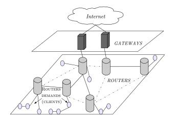
Fig. 1. An exemple of an Internet providing Wireless Mesh Network
