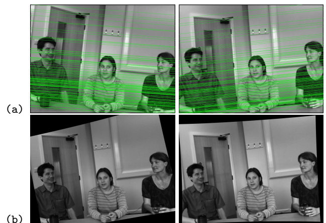
Figure 6: Visual cues: (a) original image pair with superimposed epipolar lines and (b) rectified stereo pair
