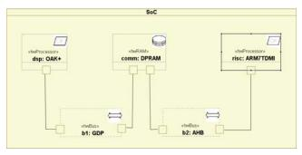
Figure 12. Modeling a hardware execution platform
