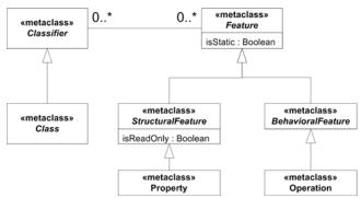
Figure 2. Meta-model of a UML classifier
