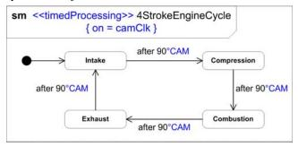
Figure 10. A state machine with multiform time
