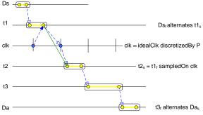
Figure 7. CCSL constraints, mixed case.
