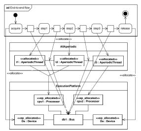
Figure 4. MARTE model, fully aperiodic case.
