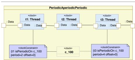
Fig. 4 Periodic threads with CCSL
