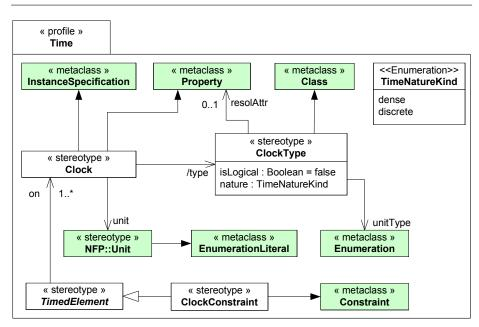
Fig. 1 Excerpt of MARTE Time subprofile
