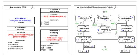
Fig. 6 Using SysML parametric diagrams
