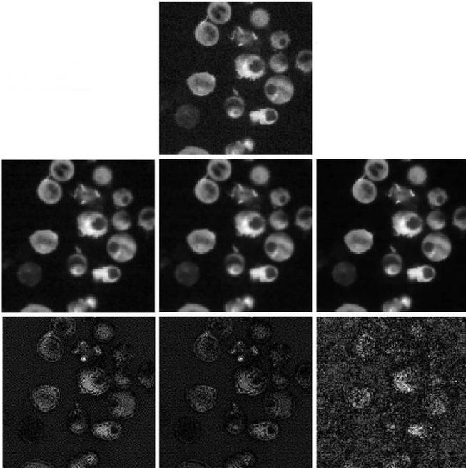
Fig. 6. Top: Noisy original image  $x$  of lymphocytes imaged by fluorescent microscopy,  $SNR = 8.14$ . Middle left: Denoised image by scalar  $TV$ ,  $SNR = 11.2$ . Middle: Denoised image by adaptive  $TV$ ,  $SNR = 12.5$ . Middle right: Denoised image  $\hat{x}$  with CS, composed from 10 images recovered with different sets of measurements,  $SNR = 14.28$ . Bottom: Images from residuals of all respective methods  $\|\hat{x} - x\|_{l_2}$ .
