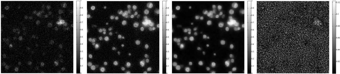
Fig. 4. Left: One noisy image  $x_i$  of drosophila cells imaged by fluorescent microscopy,  $SNR = 3.61$  and exposure time  $t = 10ms$ . Middle left: Image acquired with exposure time equal to  $t = 100ms$  and  $SNR = 6.42$ . Middle right: Denoised image  $\hat{x}$ , composed from 10 images recovered from 10 images with exposure time  $t = 10ms$ , as the first scheme proposed on Section III-B,  $SNR = 13.31$ . Right: Residual  $\|\hat{x} - I_{100ms}\|_{l_2}$ .
