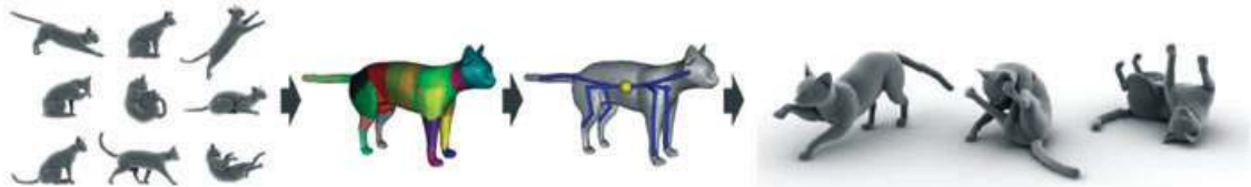
Figure 9: A set of input poses, mesh clusters representing rigid bones, computed skeleton (the yellow dot corresponds to the root of the hierarchy), and new poses created with this skeleton (Schaefer and Yuksel [SY07]).
