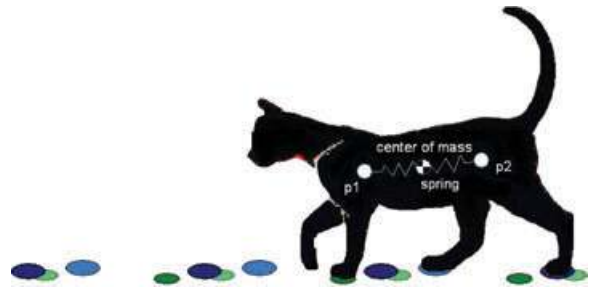
Figure 12: Two point masses are used in the simplified physics model to make the overall body movement look realistic. The footprints guide the position of the feet, the small circles represent the front legs, and the big circles represent the back legs (after [TvdP98]).
