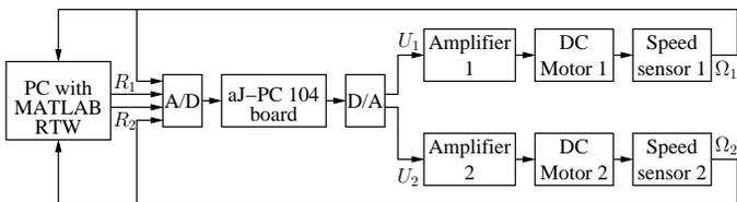
Fig. 7. Experimental setup
