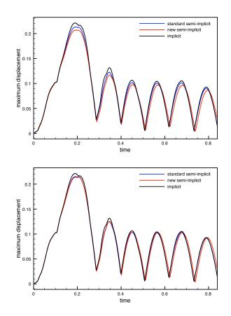
Figure 8: Comparison of the implicit, standard semi-implicit and Robin based semi-implicit coupling schemes: maximal displacement of the structure. Top: VR. Bottom: FWI.
