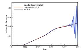
Figure 3: Comparison of the semi-implicit and Robin based semi-implicit coupling schemes: interface mid-point vertical displacement.
