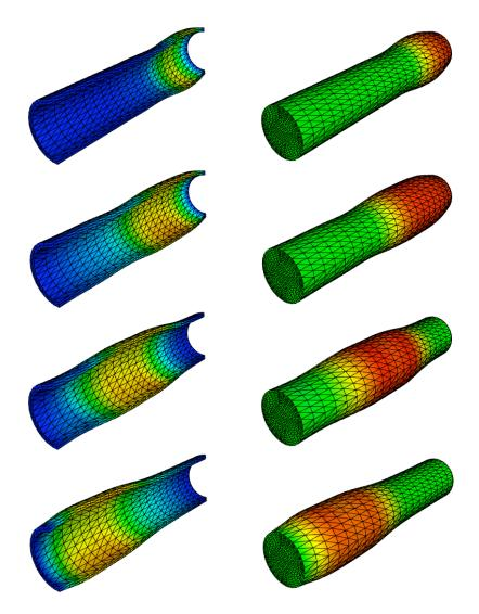
Figure 4: Robin based semi-implicit coupling: snapshots of the - exaggerated - solid deformation and of the pressure at different time instants (t = 0.0025, 0.005, 0.0075 and 0.01 seconds).
