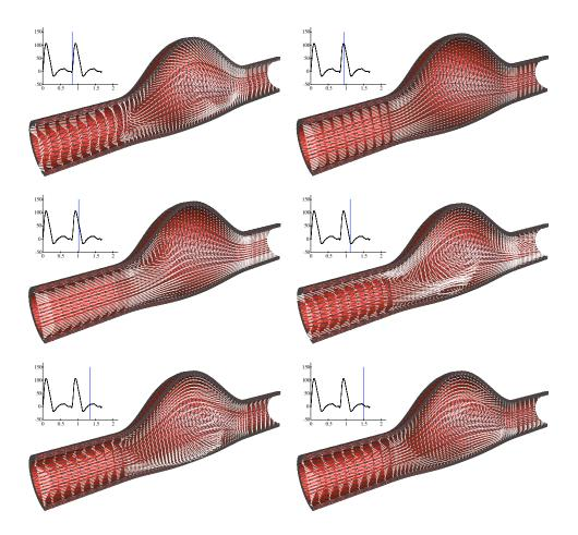
Figure 7: Robin based semi-implicit coupling: snapshots of the solid deformation and fluid velocity field at different time instants.
