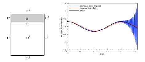
Figure 2: Left: Computational domain. Right: comparison of the semi-implicit and the Robin based semi-implicit coupling schemes (interface mid-point vertical displacement).
