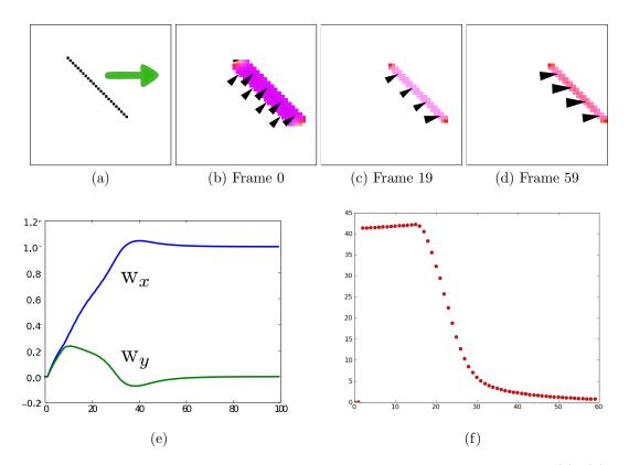
Figure 4.1: Response of the model on a horizontally translating bar presented in (a). (b)-(d) Evolution of the velocity field  $v_1(t, x)$ . (e) Temporal read-out providing a global motion similar to the one get in eye movements computed by averaging the velocity field. Green and blue correspond respectively to  $w_x$  (horizontal) and  $w_y$  (vertical) components. (f) Mean tracking error computed as the angular difference between w and the 2D translation direction of the bar.
