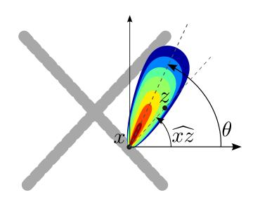
Figure 2.2: Illustration of the oriented spatial neighborhood around x in the direction  $\theta$  used to compute  $\phi_I$ . Luminosity in this oriented neighborhood is compared with the luminosity at the center.
