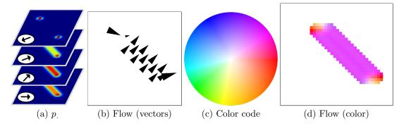
Figure 3.1: Illustration of the motion representation on the layer  $p_0$  for a translating bar. (a) Responses for the different preferred velocities. (b) Subsampled velocity field associated to distribution  $p_{.}$  shown in (a) and estimated by (3.1). (c) Middleburry color code [10] used for continuous dense output. (d) Color-based representation of the velocity field in (b).
