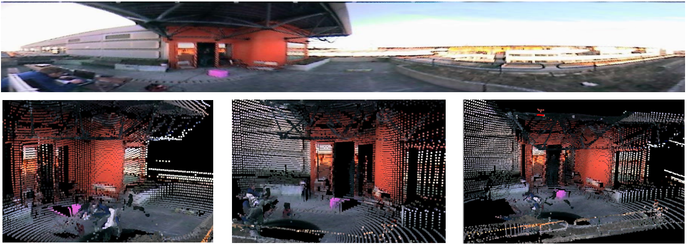
Fig. 7 The panoramic picture shown in the upper window was taken by using a hyperbolic mirror and a perspective camera, the size of 640x480 pixels. After intrinsic camera calibration, the color information was mapped onto the 3D points extracted from a sick laser range finder. In the lower windows are the mapping results. The colors are perfectly reprojected onto the 3D structure of the environment, showing that the camera calibration has been accurately done.
