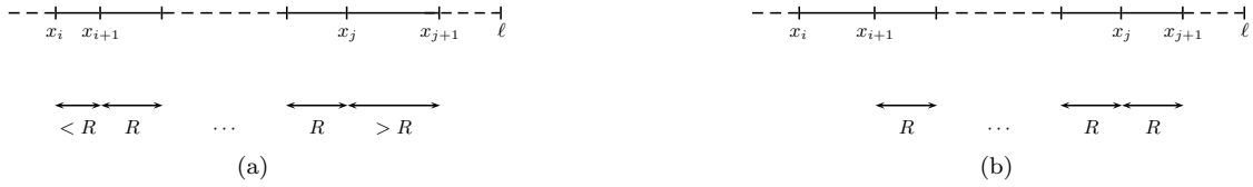
Figure 5: Impact of routing N packets from node i + 1 to node j + 1 on the network topology with respect to the segments size: s_{k+N} \geq s_k + 1 .
