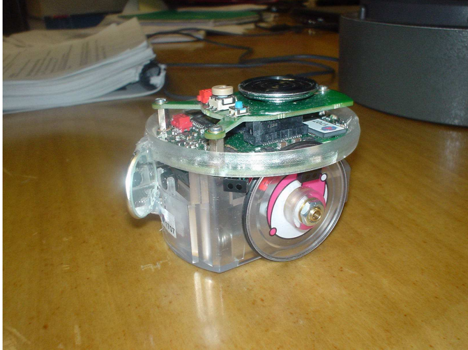
Figure 6: The robot e-puck with a small mirror in front of the camera.
