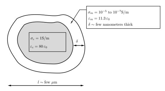
FIGURE 1. The electric model of the biological cell given by Schwan [4].
