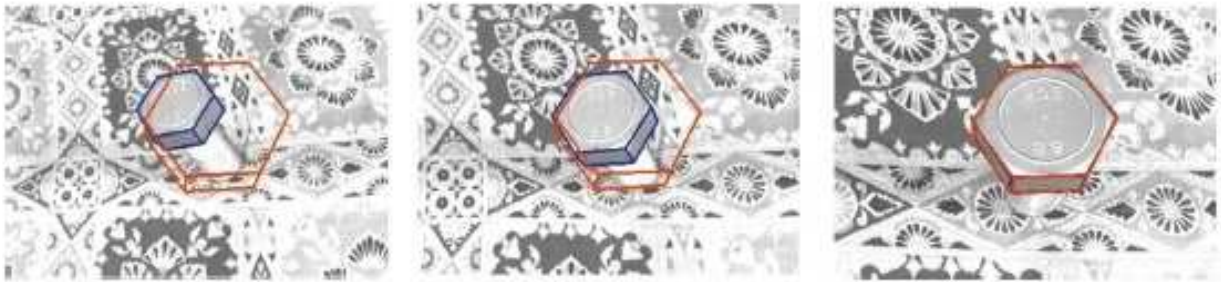
Figure 14: Positioning wrt. the nut by visual servoing within a highly textured environment at time 1, 40 and 154 (image 365 \times 256 , J = \pm 3 , \lambda = 1500 ). In red projection of the CAD model corresponding to the desired position while the projection of tracked object appears in blue.
