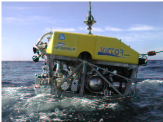
Fig. 1. The Ifremer Victor 6000 underwater ROV (© Ifremer)
