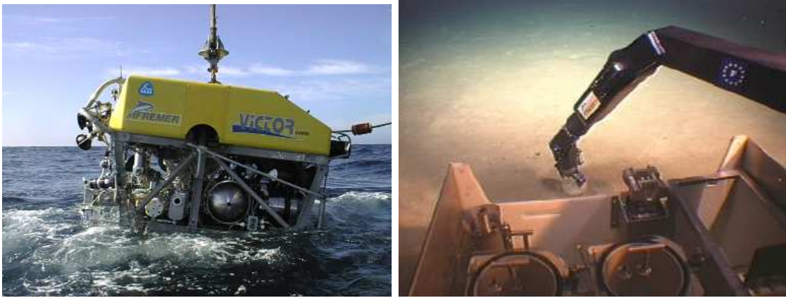
Figure 1: The Ifremer Victor 6000 underwater ROV and its 6 dof Maestro manipulator (© Ifremer)
