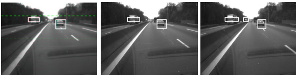
Figure 3. Obstacle detection and tracking in a highway environment
