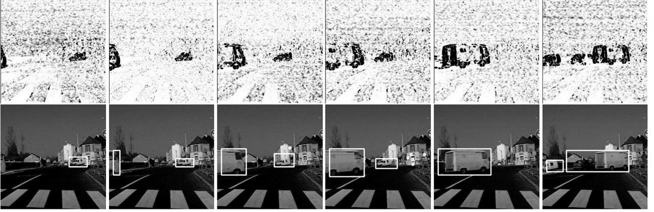
Figure 1. Obstacle detection from a motionless vehicle. The first and third rows display the outliers maps, the second and fourth rows contains the detected obstacles (see text for details)
