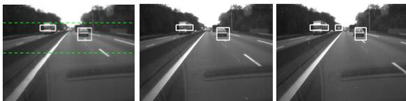
Figure 3. Obstacle detection and tracking in a highway environment
