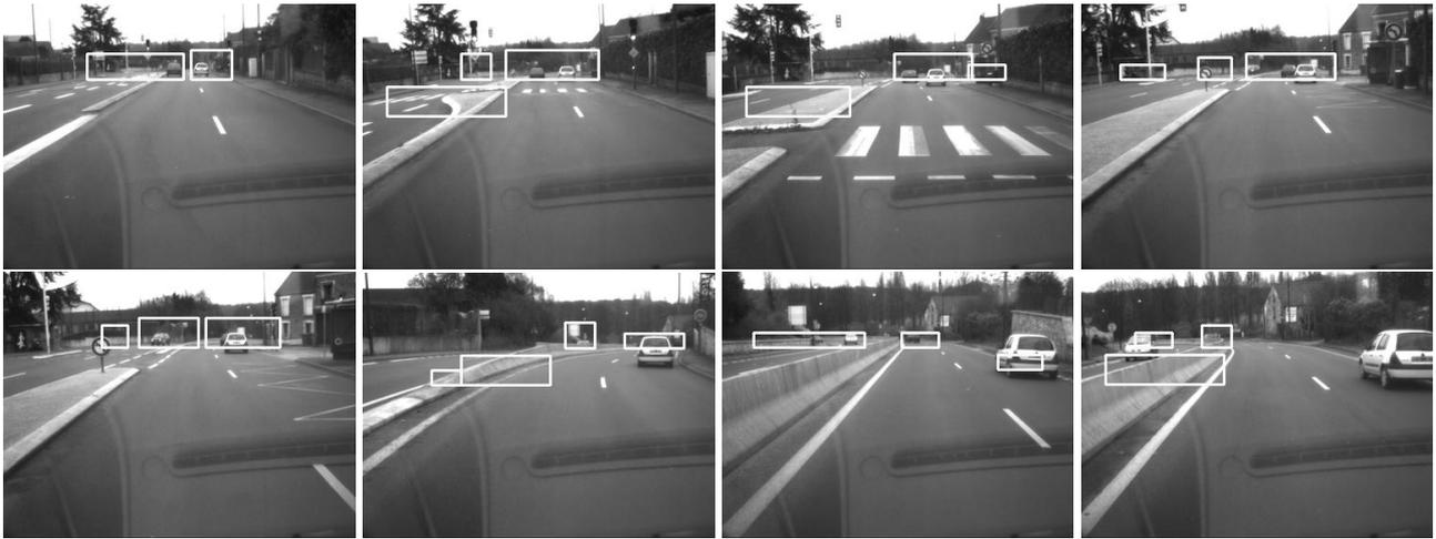
Figure 4. Detection of multiple (moving and static) obstacles in a road environment.
