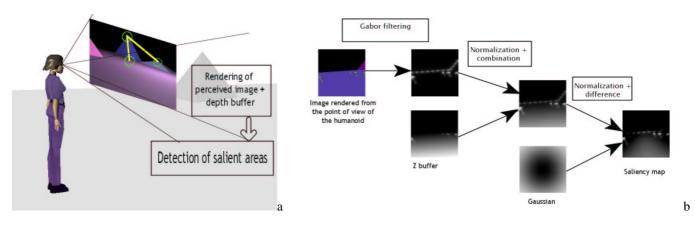
**Fig. 1**. (a) Using saliency map to perceive the environment. Green circles are conspicuous zones, and the yellow lines are a pathway between those zones (b) obtaining a saliency map based on spatial frequencies and depth information
