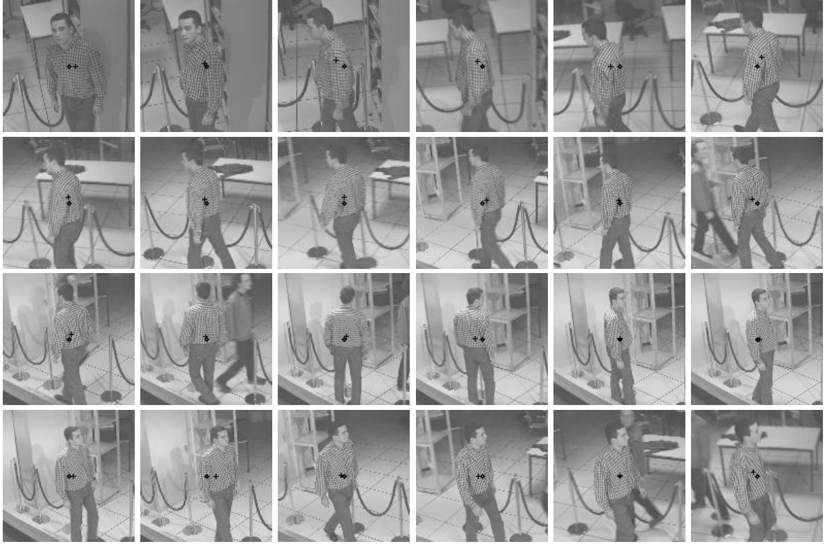
Fig. 7. Tracking of a pedestrian. An image upon ten of the acquired sequence (approximately 2 frames per second). Cross (+) stands for the estimated c.o.g. and diamond (◊) for the image center
