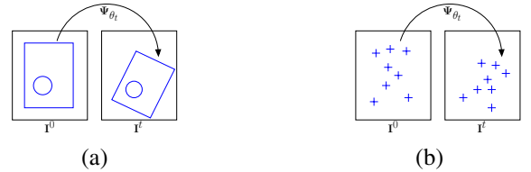
Fig. 2. (a) Estimating the object motion using edge information, (b) Estimating the object motion using texture information
