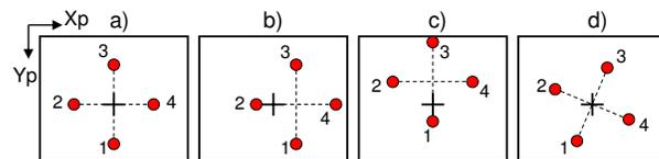
Fig. 2. Effects of laser-cross misalignment in the desired image. a) Ideal image. b) The laser-cross is horizontally displaced or rotated around  ${}^C Y$ . c) The laser-cross is vertically displaced or rotated around  ${}^C Y$ . d) Laser-cross rotated around  ${}^C Z$ .
