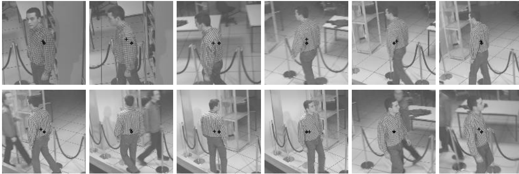
Figure 8. Tracking of a pedestrian. An image upon ten of the acquired sequence (approximately 2 frames per second). Cross (+) stands for the estimated c.o.g. and diamond (◊) for the image center
