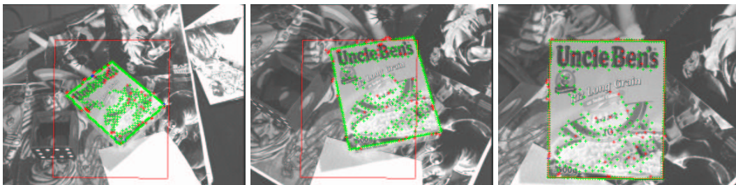
Figure 6. Hybrid tracking: merging contour and appearance within a single non-linear minimization process.
