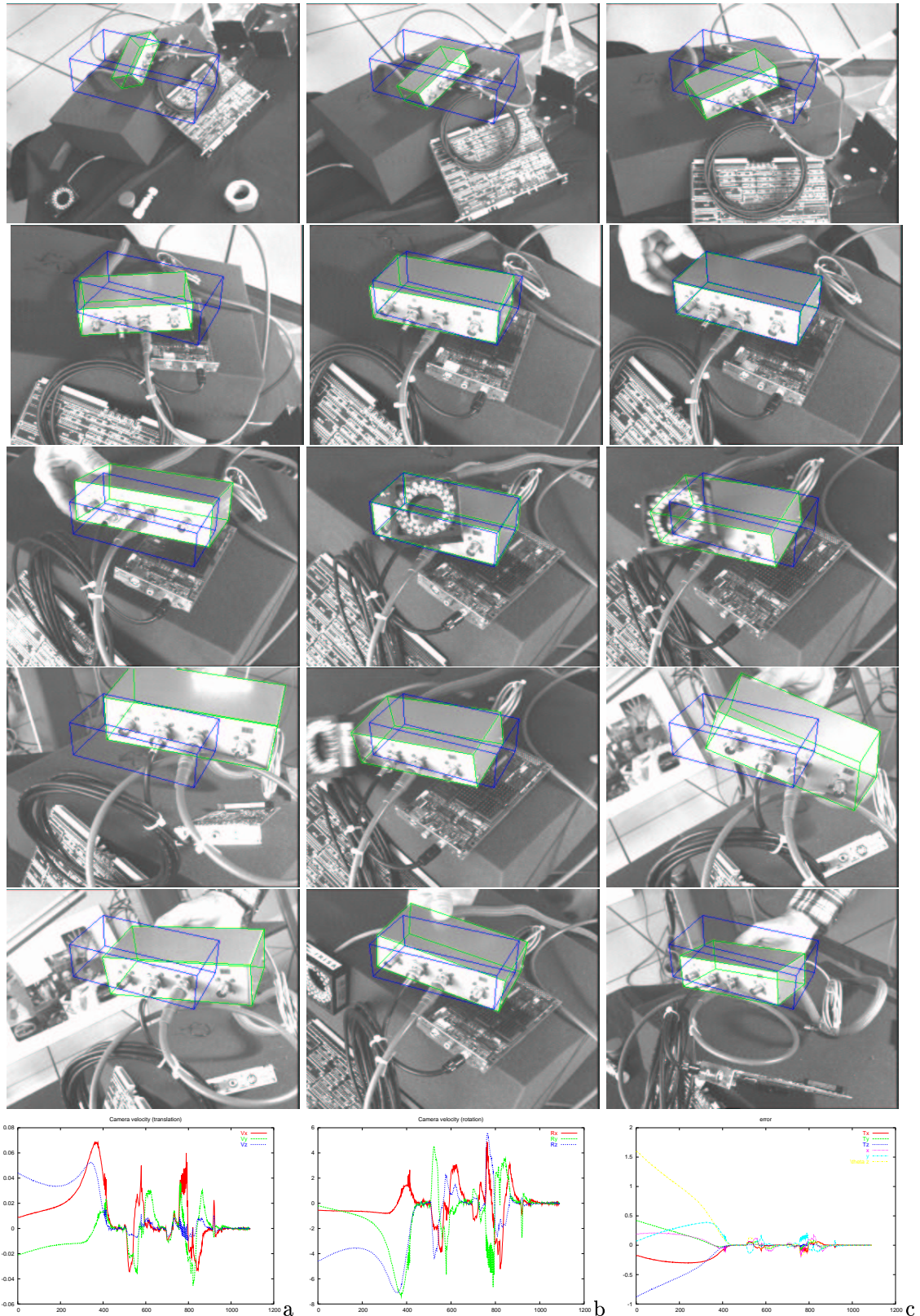
Figure 5: 2D 1/2 visual servoing experiments. The six first images have been acquired in initial visual servoing step. In the reminder images object is moving along with the robot (a-b) camera velocity in rotation and translation (c) error vector \mathbf{s} - \mathbf{s}^* . Images are acquired and processed at frame rate (50Hz).
