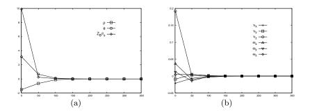
Fig. 10. Modeling error  $\hat{R} = 5R$ : (a)  $\mathbf{s}_{\mathbf{p}}$  error; (b) computed camera velocities (m/s and dg/s)
