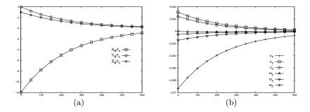
Fig. 7. Modeling error  $\widehat{R} = 0.2R$ : (a) s error; (b) computed camera velocities (m/s and dg/s)
