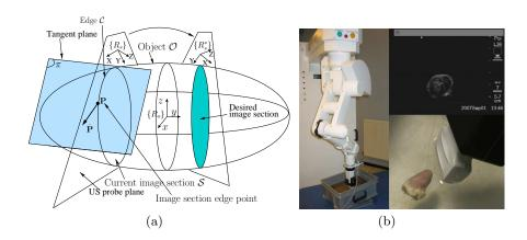
**Fig. 1.** (a) Interaction between the ultrasound probe and the object - (b) Experimental setup: (left) ultrasound probe mounted on a 6 DOF medical robot - (right) Observed US image and the rabbit heart suspended in a water-filled box
