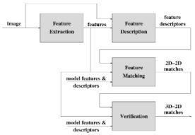
Figure 4: On-line Object Recognition
