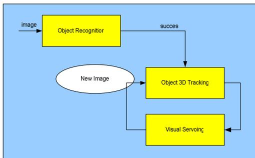
**Figure 1:** For Vision Based Manipulation of a non-cooperative object three steps are required: Object Recognition, Object Tracking and Visual Servoing
