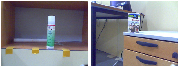
Fig. 3. Panoramic-based arm positioning: images acquired by the embedded camera before and after the motion.
