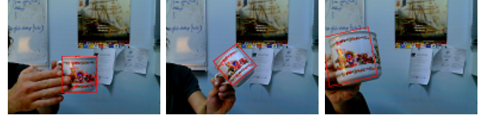
Fig. 8. Cup tracking. Only the right image is shown. The first view is the initial one where the box has been defined.
