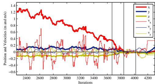
Fig. 4. Experiment B: Position and velocity of the object in the gripper frame, obtained after Kalman filtering. The two components  $x$  and  $y$  are regulated to 0 thanks to the task  $e_\theta$ . The last component  $z$  slowly decreases to 0 while walking, and is finally regulated to 0 from iteration 3700 when the task  $e_{3D}$  is introduced in the stack.
