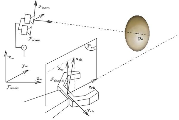
Fig. 1. Definition of frames  $\mathcal{F}_{rhand}$  and  $\mathcal{F}_{licam}$ .
