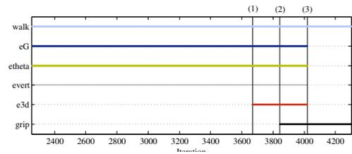
Fig. 2. Experiment B: Activation of the task in the stack during servo. At the beginning of the servo, the tasks  $e_{walk}$ ,  $e_G$ ,  $e_{vert}$  and  $e_\theta$  are in the stack. At Event (1) (Iteration 3650), the task  $e_{3d}$  is put in the stack to grasp the object. The object is in the gripper from Event (2) (Iteration 3800). The gripper closure starts. All the tasks are removed from the stack as soon as the gripper is close on the object, at Event (3) (Iteration 4000).
