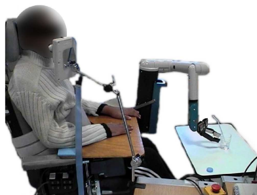
Fig. 3. The AVISO system consists of a MANUS arm [17], [33] mounted on a wheelchair, a stereo vision system fixed on the end effector of the arm, a graphical interface displayed on a monitor, any device adapted to the user's handicap (speech recognition, head movement, breath controller, joystick, etc. )
