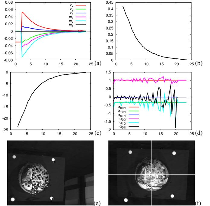
Fig. 2. 1<sup>st</sup> experiment ( $x$  axes in seconds).  ${}^d\Phi = 0$ . (a) Kinematic screw (m/s or rad./s). (b) Error defined as  $\|e\|$ . (c) Magnitude of the rotation  $\theta$  (deg.) (d) Vector  $\alpha$  in a fixed frame (filtered and non-filtered). (e) Initial image. (f) Final image.
