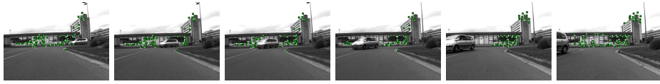
Fig. 7. Images obtained during the execution of a navigation experiment. The points used for navigation re-appear after being occluded and disoccluded by a moving car.
