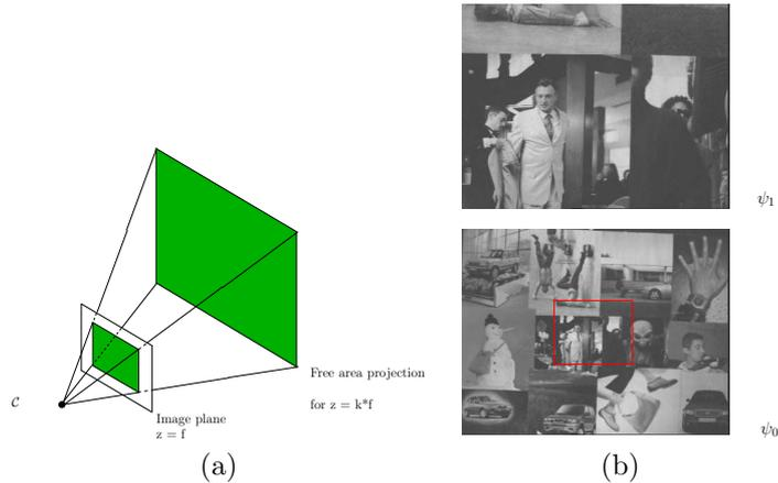
Figure 5: Motions along the optical axis: (a) visibility cone associated with free area  $\mathcal{I}_{free}$ , (b) comparing the image borders after a motion along the optical axis
