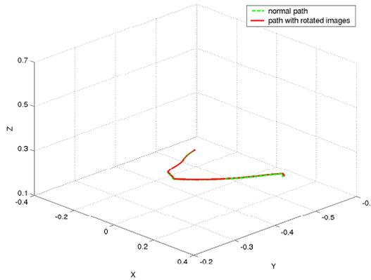
Figure 23: Exp. 4: Robot trajectories compared (path defined by Fig. 19 and the same with rotated images). The two trajectories are equivalent, since the robotic system uses the feature positions in the current frame to control its motion, and not the one observed within the images from the path. The rotated images do not disturb the control law.
