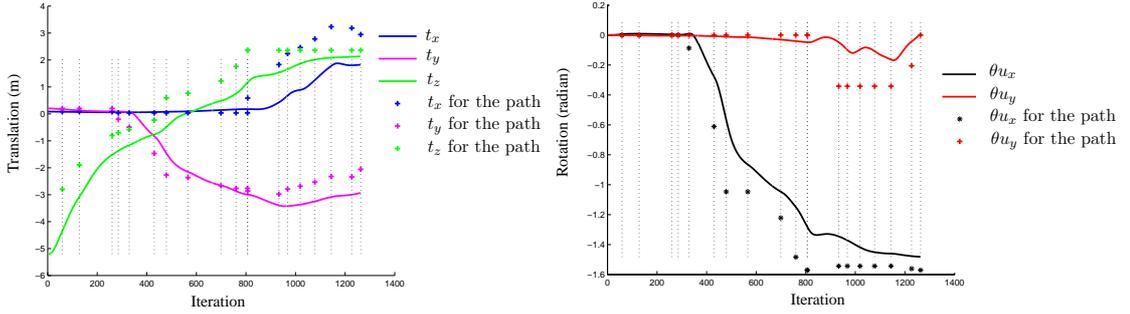
Figure 14: Exp. 1: Position of the camera (translation and orientation) during the navigation. Vertical lines indicate a change of interest set  $\mathcal{M}_i$  used to control the system. Crosses indicate the pose associated to the view  $\psi_{i+1}$  of the set  $\mathcal{M}_i$  just before the change of interest set. The robotic system does not converge towards each of these positions.
