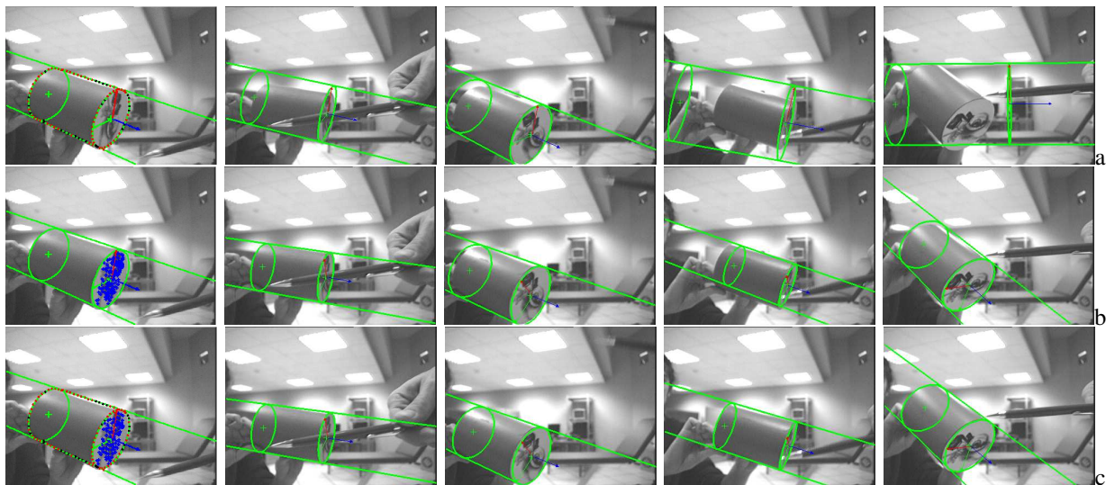
Fig. 5. Cylinder sequence. Images for (a): the edge-based tracker, (b): the texture-based one, (c): the hybrid one. The hybrid tracker is the better one, despite the specularities and the misleading environment. For the initial images, the grey level samples are represented by blue crosses and the edge location by red points if an edge is detected or a black one otherwise
