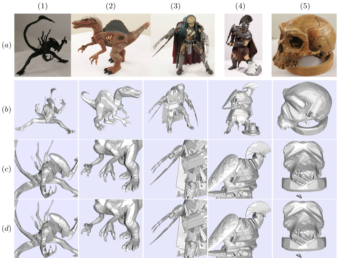
Fig. 14. (a) Original models. (b) Reconstruction obtained with dense subpixel contours using our algorithm (EPVH). (c) Close up of dense contour reconstruction. (d) Same close-up using image-resolution silhouette bitmaps: reconstructions are less smooth but carry the same surface information, hardly distinguishable from their subpixel input counterparts. (1) Alien: 24 views, 1600 \times 1600 . (2) Dinosaur: 24 views, 2000 \times 1500 . (3) Predator: 1800 \times 1700 . (4) Roman: 48 views, 3500 \times 2300 . (5) Skull: 1900 \times 1800 . All five datasets courtesy Lazebnik, Furukawa & Ponce.
