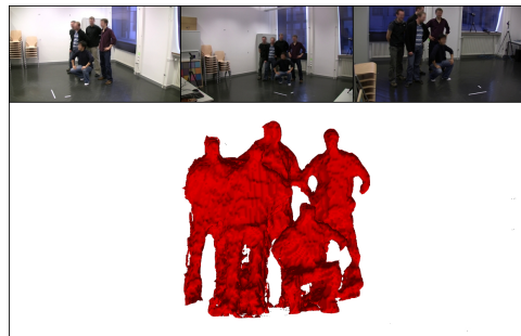
Figure 13. The reconstruction of the densely populated scene from all 9 sensors with concavity and details. Visual hull fails in this case, resulting an indistinguishable blob.
