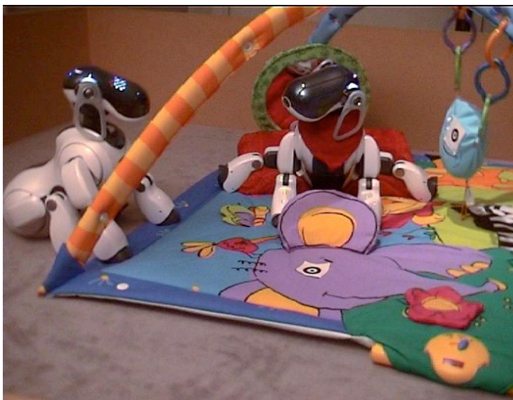
Figure 5: A four-legged robot is placed on a playmat. The robot can move its arms, its neck and its mouth and can produce sound. Various toys are placed near the robot, as well as a pre-programmed “adult” robot which can respond vocally to the other robot in certain conditions.
