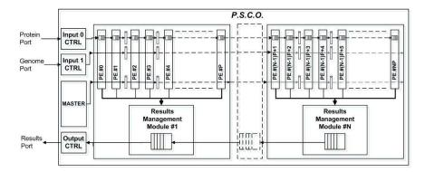
Figure 2: PSC Operator Arcitecture
