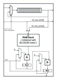
Figure 3: Processing Element Architecture
