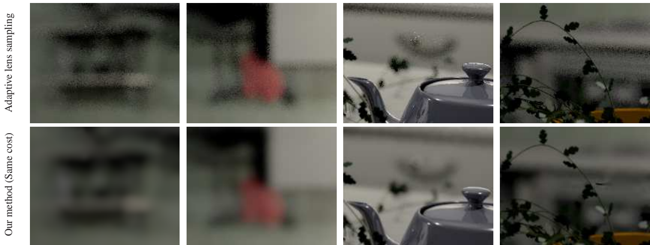
Fig. 10: Comparison between our method (bottom row) and adaptive lens sampling based on variance estimation from a small number of samples (top row). Both methods use the same total number of primary rays for the entire image. While the adaptive lens sampling manages to uniformize the variance across the image, it needs to send rays for each and every pixel while our method only samples a few pixels in the most blurry regions. This makes the adaptive lens sampling unable to compete with our method at equal number of primary rays. This explains why the images are noisier than the ones produced using our method.
