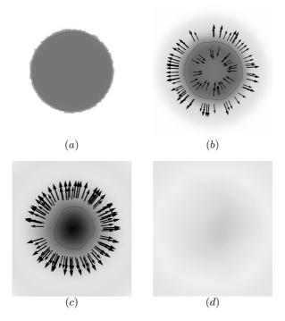
**Fig. 4.** On this four figures, the density is in grey-scale: the higher is the darker; the velocity is shown with arrows, and the bubble is represented with an iso of the volume fraction. At the beginning, a bubble of liquid is inside a gas (a). The liquid is metastable, which induces a phase transition front, and sonic waves: a shock is emitted inside (b), then focus in the center of the bubble (c). Last, the bubble disappears (d), and behaves as a single phase problem which goes at rest.
