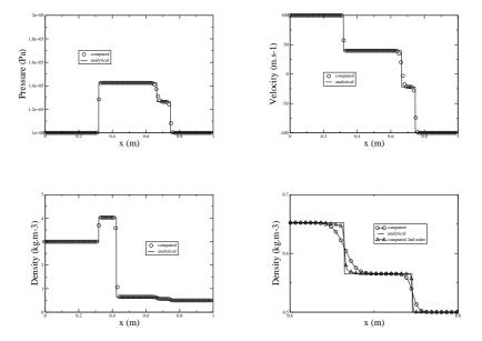
**Fig. 3.** Comparison of the numerical solution obtained and the analytical one for a shock splitting, for density, pressure and velocity. The last figure is a zoom on the split shock, in which we compare the first and second order computed solutions.
