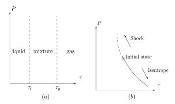
**Fig. 1.** (a): The thermodynamic plane is divided into three zones in which either a pure phase (liquid or gas) is stable, or a mixture is stable. On the lines  $\tau = \tau_i$ , the equation of state is continuous, but cannot be differentiated. (b): A wave curve in the thermodynamic plane  $(\tau, P)$  is a decreasing curve. Under the initial state, the wave curve is an isentrope, whereas above, the wave curve is a shock.
