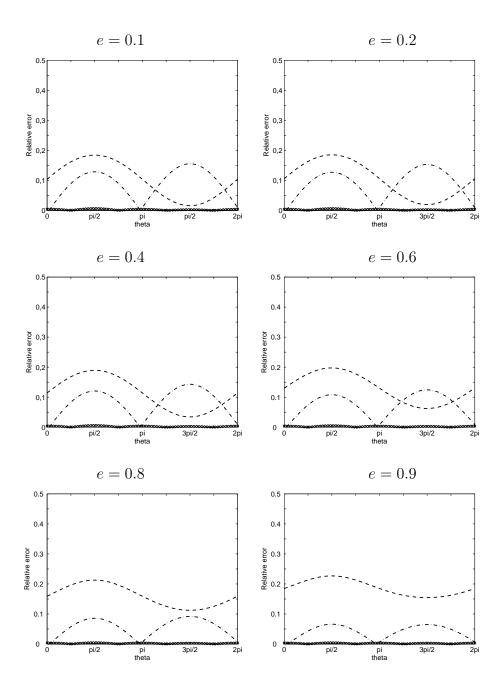
Fig. 5. Relative error of the specific impedance corresponding to DtN1 (dashed/dotted), DtN2 (crossed), BGT2 (dashed) when solving two-dimensional sound-soft scattering problem with ka = 0.1 and incident angle  $\theta_0 = \frac{\pi}{2}$  (The relative error for DtN2 is below 2%).
