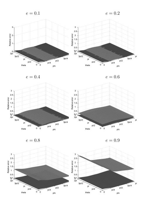
Fig. 16. Relative error of the specific impedance corresponding to DtN2 (black) and BGT2 (dark grey) when solving three-dimensional sound-soft scattering problem with ka = 1 and incident angle  $\varphi_0 = 0$ .
