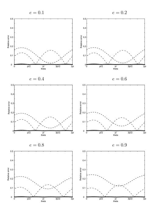
Fig. 4. Relative error of the specific impedance corresponding to DtN1 (dashed/dotted), DtN2 (crossed), BGT2 (dashed) when solving two-dimensional sound-soft scattering problem with ka = 0.1 and incident angle  $\theta_0 = \frac{\pi}{4}$  (The relative error for DtN2 is below 2%).
