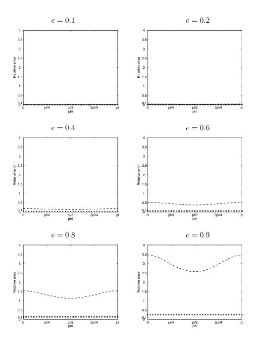
Fig. 11. Relative error of the specific impedance for DtN2 (crossed), BGT2 (dashed) when computing the prolate spheroidal mode (m, n) = (1, 1) for ka = 0.1.
