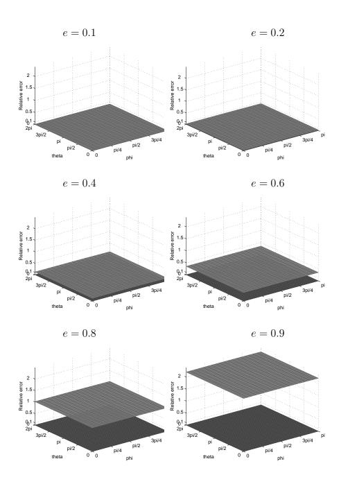
Fig. 15. Relative error of the specific impedance corresponding to DtN2 (black) and BGT2 (dark grey) when solving three-dimensional sound-soft scattering problem with ka = 0.1 and incident angle  $\varphi_0 = \frac{\pi}{2}$ .
