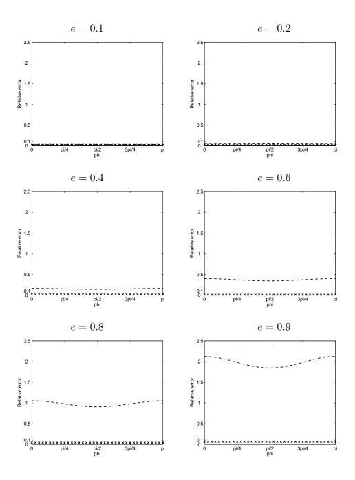
Fig. 10. Relative error of the specific impedance for DtN2 (crossed), BGT2 (dashed) when computing the prolate spheroidal mode (m, n) = (0, 2) for ka = 1.
