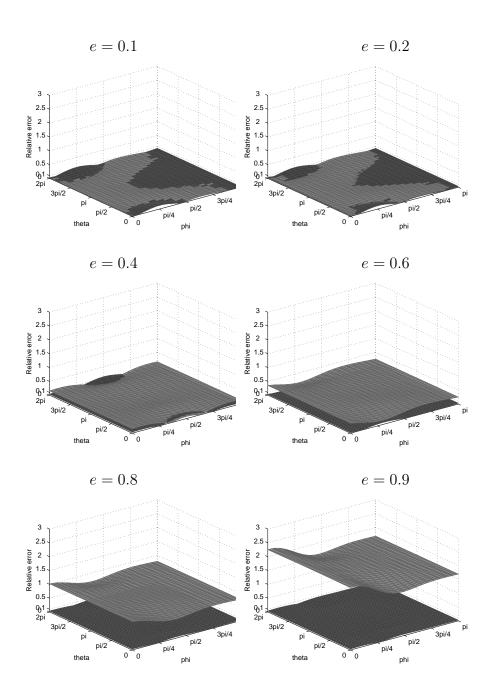
Fig. 17. Relative error of the specific impedance corresponding to DtN2 (black) and BGT2 (dark grey) when solving three-dimensional sound-soft scattering problem with ka = 1 and incident angle  $\varphi_0 = \frac{\pi}{4}$ .
