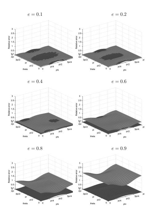
Fig. 18. Relative error of the specific impedance corresponding to DtN2 (black) and BGT2 (dark grey) when solving three-dimensional sound-soft scattering problem with ka = 1 and incident angle  $\varphi_0 = \frac{\pi}{2}$ .
