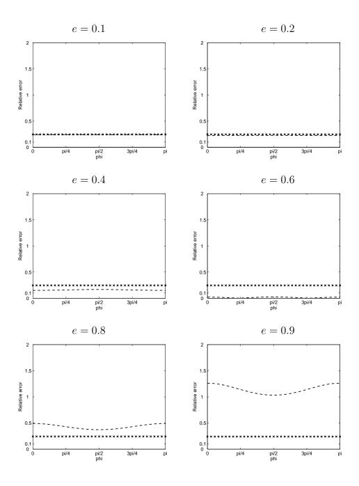
Fig. 9. Relative error of the specific impedance for DtN2 (crossed), BGT2 (dashed) when computing the prolate spheroidal mode (m, n) = (0, 2) for ka = 0.1.
