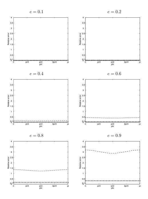
Fig. 12. Relative error of the specific impedance for DtN2 (crossed), BGT2 (dashed) when computing the prolate spheroidal mode (m, n) = (1, 1) for ka = 1.
