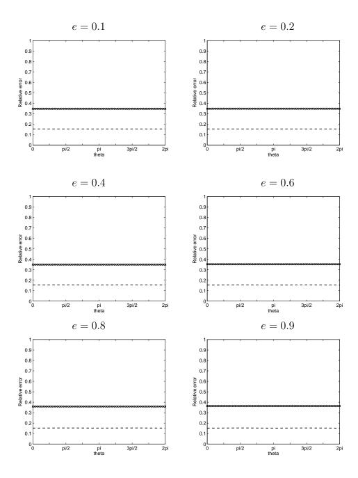
Fig. 1. Relative error of the specific impedance for DtN2 (crossed), BGT2 (dashed) when computing the second *even* elliptical mode (n = 2) for ka = 0.1.
