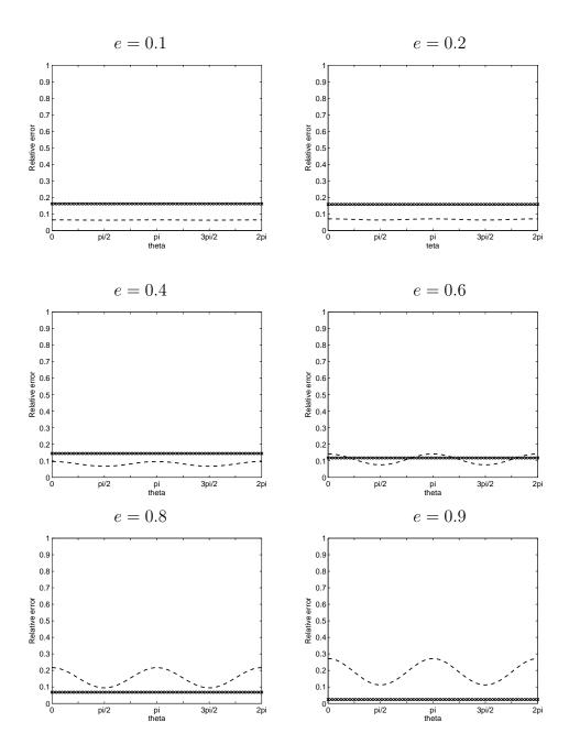
Fig. 2. Relative error of the specific impedance corresponding to DtN2 (crossed), BGT2 (dashed) when computing the second *even* elliptical mode (n = 2) for ka = 1.
