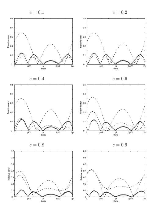
Fig. 7. Relative error of the specific impedance corresponding to DtN1 (dashed/dotted), DtN2 (crossed), BGT2 (dashed) when two-dimensional solving sound-soft scattering problem with ka = 1 and incident angle  $\theta_0 = \frac{\pi}{4}$ .
