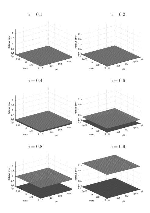
Fig. 14. Relative error of the specific impedance corresponding to DtN2 (black) and BGT2 (dark grey) when solving three-dimensional sound-soft scattering problem with ka = 0.1 and incident angle  $\varphi_0 = \frac{\pi}{4}$ .
