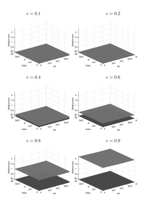
Fig. 13. Relative error of the specific impedance corresponding to DtN2 (black) and BGT2 (dark grey) when solving three-dimensional sound-soft scattering problem with ka = 0.1 and incident angle  $\varphi_0 = 0$ .
