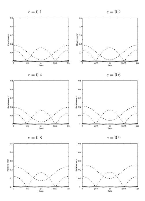
Fig. 3. Relative error of the specific impedance corresponding to DtN1 (dashed/dotted), DtN2 (crossed), BGT2 (dashed) when solving two-dimensional sound-soft scattering problem with ka = 0.1 and incident angle  $\theta_0 = 0$  (The relative error for DtN2 is below 2%).
