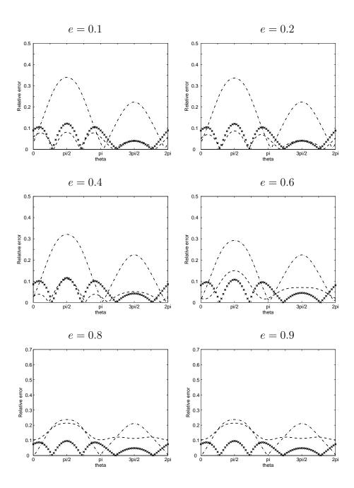
Fig. 8. Relative error of the specific impedance corresponding to DtN1 (dashed/dotted), DtN2 (crossed), BGT2 (dashed) when solving two-dimensional sound-soft scattering problem with ka = 1 and incident angle  $\theta_0 = \frac{\pi}{2}$ .
