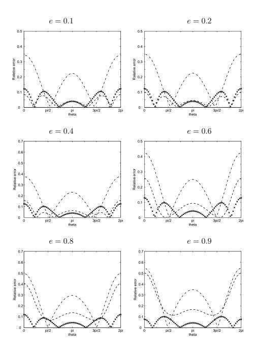
Fig. 6. Relative error of the specific impedance corresponding to DtN1 (dashed/dotted), DtN2 (crossed), BGT2 (dashed) when solving two-dimensional sound-soft scattering problem with ka = 1 and incident angle  $\theta_0 = 0$ .
