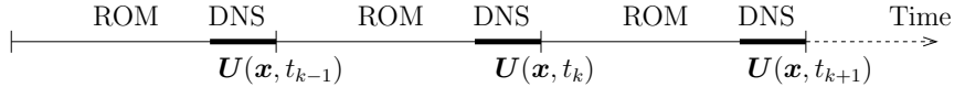
Fig. 24. Schematic representation of the hybrid method DNS-POD ROM to improve the POD subspace.
