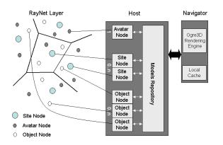
Figure 2: Nodes hosted on a proxy server to allow accesses to the metaverse on terminals with low resources such as mobiles.
