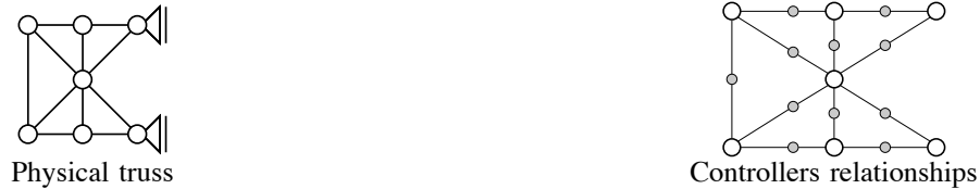
Fig. 4. On the left, a simple truss. On the right, the corresponding cells: beam and joint cells are represented respectively by big white discs and little gray discs. The edges shows the neighbourhood relationships.
