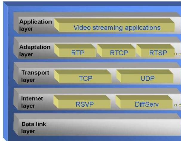
Figure 2: Video transmission: Solutions positioning over Internet architecture
